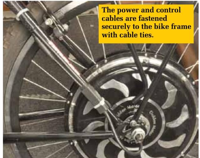
Also tighten any cable ties fully and snip their ends off, mainly for neatness but also to ensure that any ends don't interfere with brakes or any of the controls. And it's better to have too many cable ties than not enough.
