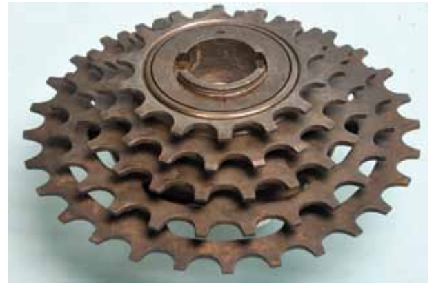
They call them gear cassettes – this one came off the original wheel and was easily fitted to the new (powered) wheel – it simply screws on.
