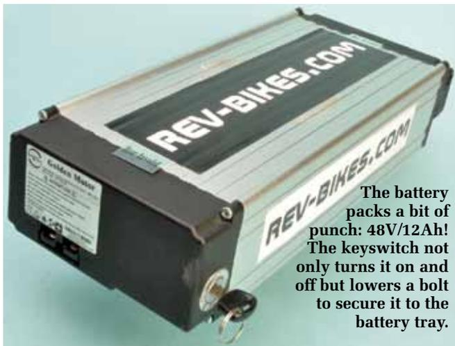
The battery packs a bit of punch: 48V/12Ah! The keyswitch not only turns it on and off but lowers a bolt to secure it to the battery tray.
