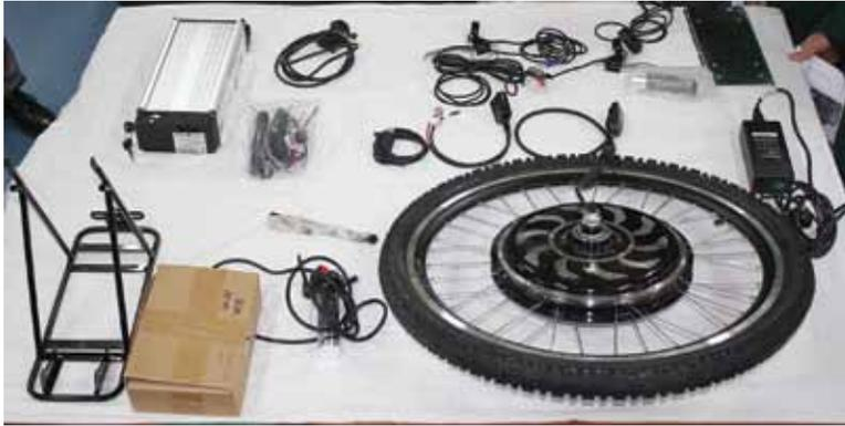
Lay out all components on a table or clean floor to check that you have everything. Here the tube/tyre is already fitted and there are some differences between this kit (the Mater Maria kit) and the one we used. At right is a shot inside the “Magic Pie” motor, which also shows the integrated controller.
