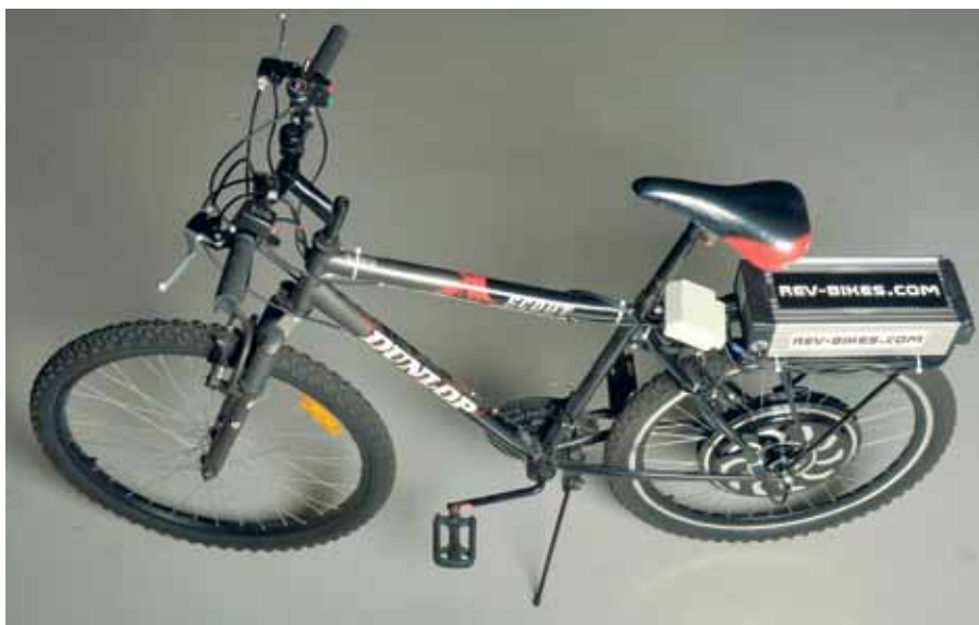
The finished eBike. Apart from tightening the spokes, total time to complete was only a couple of hours. It's still a standard mountain bike (albeit several kilos heavier!) which can be ridden normally if the battery goes flat.
