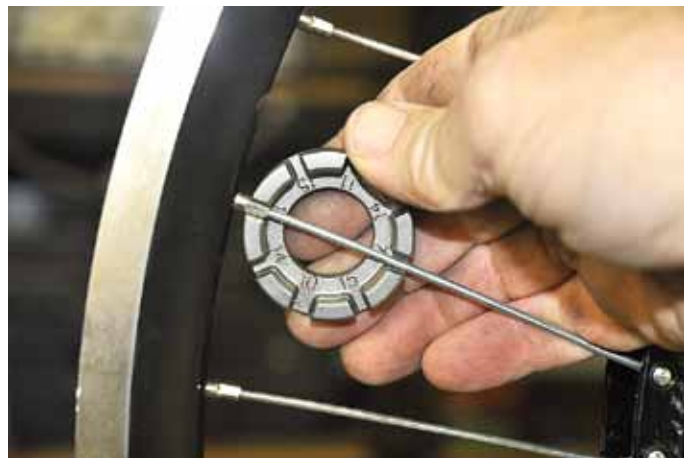
The spokes are usually loose to prevent warping in transit. A $6 spoke key soon had them nice and tight.
